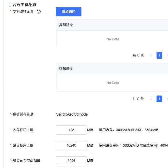
The screenshot shows the '容灾主机配置' (Disaster Recovery Host Configuration) section. It includes two main sections: '复制路径设置' (Copy Path Configuration) and '容灾主机配置' (Disaster Recovery Host Configuration). Under '容灾主机配置', there are four configuration items:
